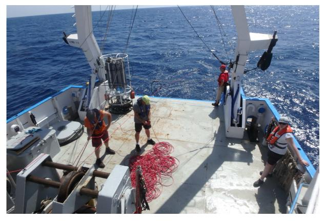
Retrieving of the *Biospherical* C-OPS (Compact-Optical Profiling System) after its deployment at the BOUSSOLE site
